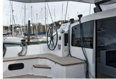
Out in the cockpit, the dual helm stations are positioned behind the saloon bulkhead, centralising weight and reducing motion, as well as giving you protection from the elements. You can sit on the coaming or stand at the wheel for excellent vision all-round, with the main and jib sheets positioned right in front of you and the traveller and spinnaker sheets close to hand.
