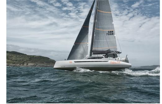
Out on the fore deck one can feel the power of this boat, with its striking bows and carbon spinnaker pole projecting forward, and know this is a thoroughbred machine. The simplicity of its engineering and lack of forward beam means the bows can be driven fast through waves without tripping over the beam and causing so much spray that it makes life in the cockpit unbearable.
