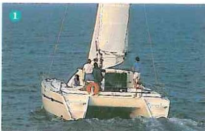
1 *The Lagoon 37 is crafted in hand laid up fiberglass with balsa coring for stiffness, strength, insulation and of course, outstanding performance.*
